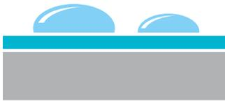
The **EVERCARE™** water-repellent effect prevents staining products from penetrating the materials (alcohol-based Eosin and Betadine, hydro-alcoholic gels, etc.), remaining on the surface.
