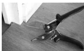
Mitre shears Reference : Romus : 93415 / Janser : 237 530 000 For cutting around door frame bases and areas which are difficult to access.
